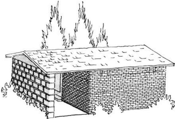
SECOND ALTERNATE shows the cement block faced with bricks. Use one course 4-inch brick and two courses of 8-inch cement block to obtain the required weight per unit area.
