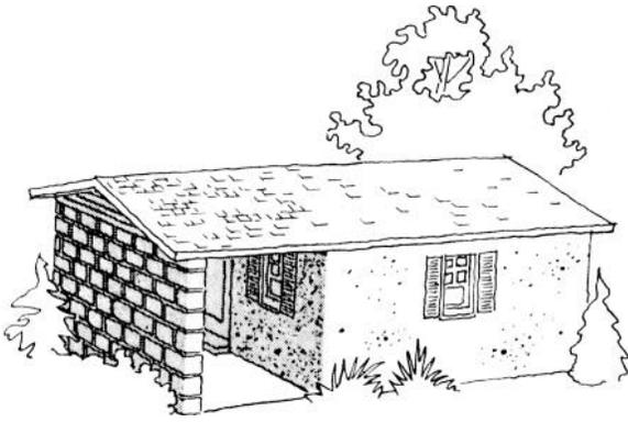
FIRST ALTERNATE indicates windows in the workshop area. Solid blocks, equal to a thickness of 12 inches, should be available to fill these openings to provide adequate fallout protection. Window sizes should be kept small. When using the shelter for protection against high winds, do not place the concrete blocks in the doorway or windows.
